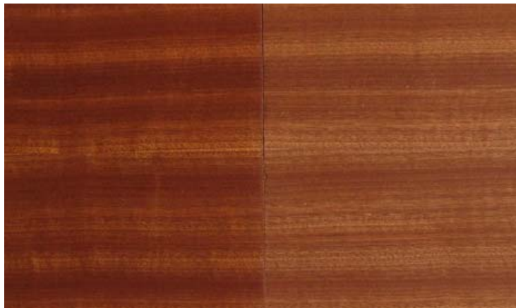
Left: first coat with UV-PUD 4. Right first coat with UV-PUD 1
