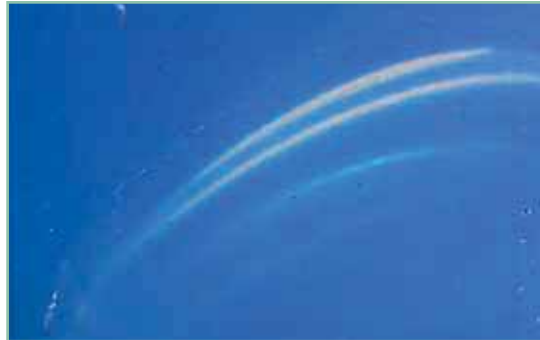
Excellent pigment stabilization "rub out test"
