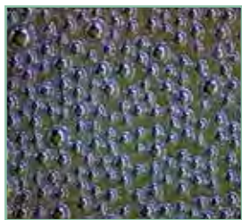
Micro foam bubbles in a solvent-borne clear coat
