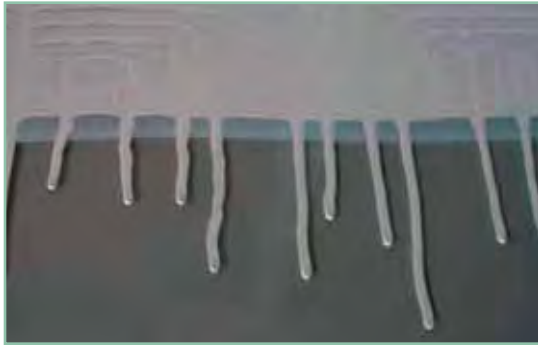
Sagging of paint on vertical substrate
