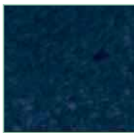
Closed surface obtained with ADDITOL XW 6544
