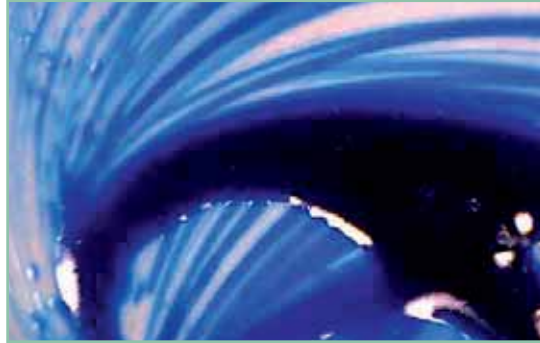
Strong pigment floating visible "rub out test"
